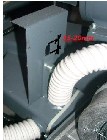
Figure 17. Position of max. opening of vent. flap
