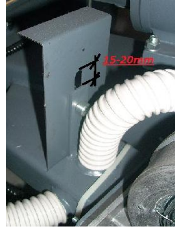
Figure 14. Position of fan flap.
