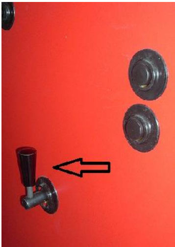
Figure 15. Position of flap handle for- INITIATING FIRE
