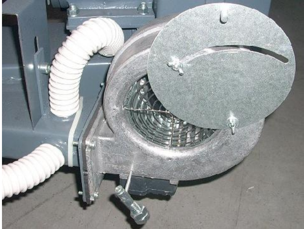
Figure 13. Position max. open of the fan flap
