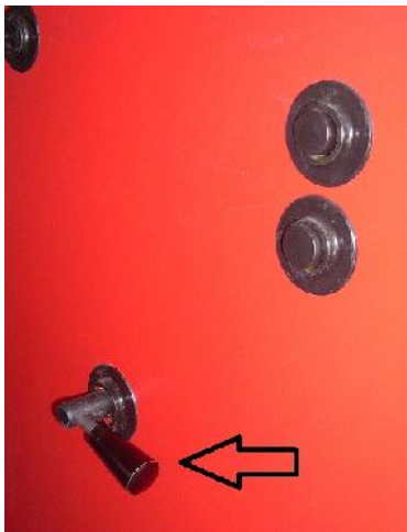
Figure 17. Position of flap handle (working position)
