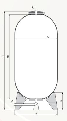
A - Inlet B - Outlet \* up to 5 connections each
