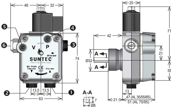
Inlet ① and Return ② with direct sealing for revision 6 models (sealing with washers can also be used)
