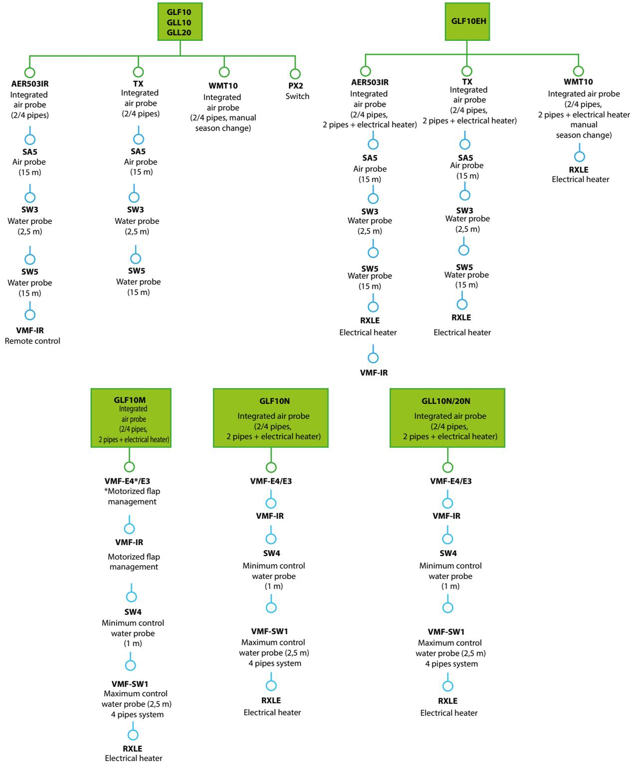
**RXLE it can be installed only at the factory.**
